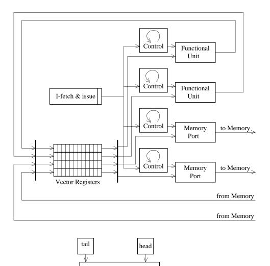
Counter-based control allows very fast clock (e.g. 2X normal scalar clock)
